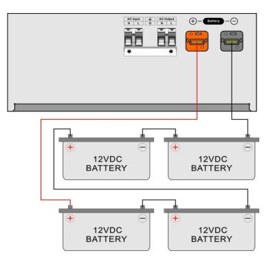
5.4 Input/Output wiring diagram
