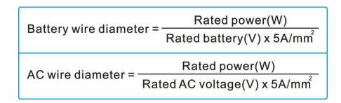
For example: Wire diameter of 5000W/48Vdc/220Vac as below:
